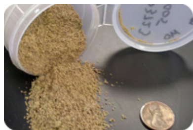
Metals free, powdered bark sample after ground with Knife Mill
