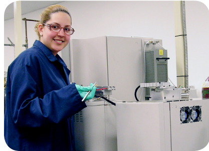
LECO TruSpec CHNS Analyzer with Oxygen Module
