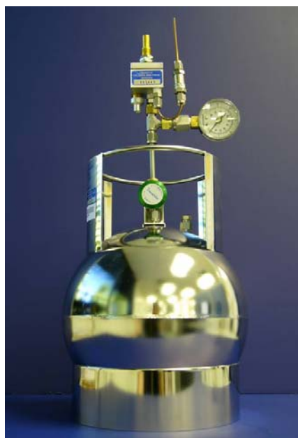
Figure 3. Detailed photograph of stainless steel canister, analog vacuum gauge, and flow controller.
