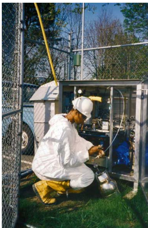
Figure 2. Photograph of EPA TO-15 sampling with stainless steel canister.
