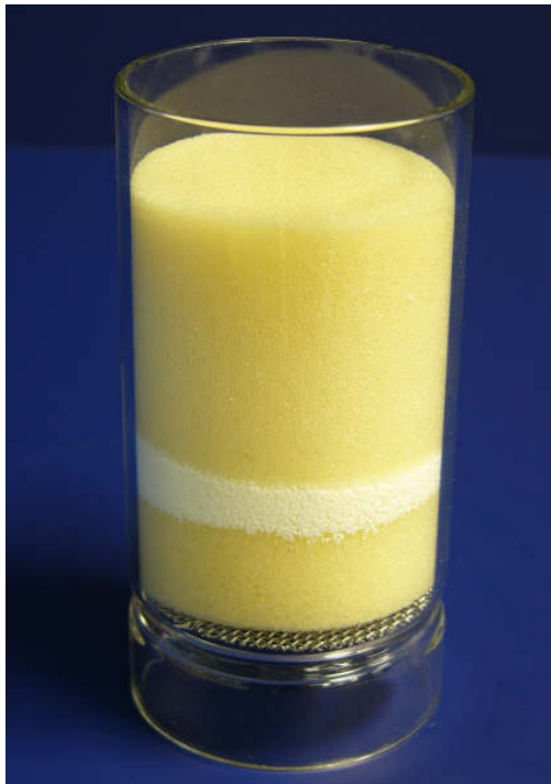
Figure 5. Detailed photograph of high volume PUF/XAD sampling media cartridge.
