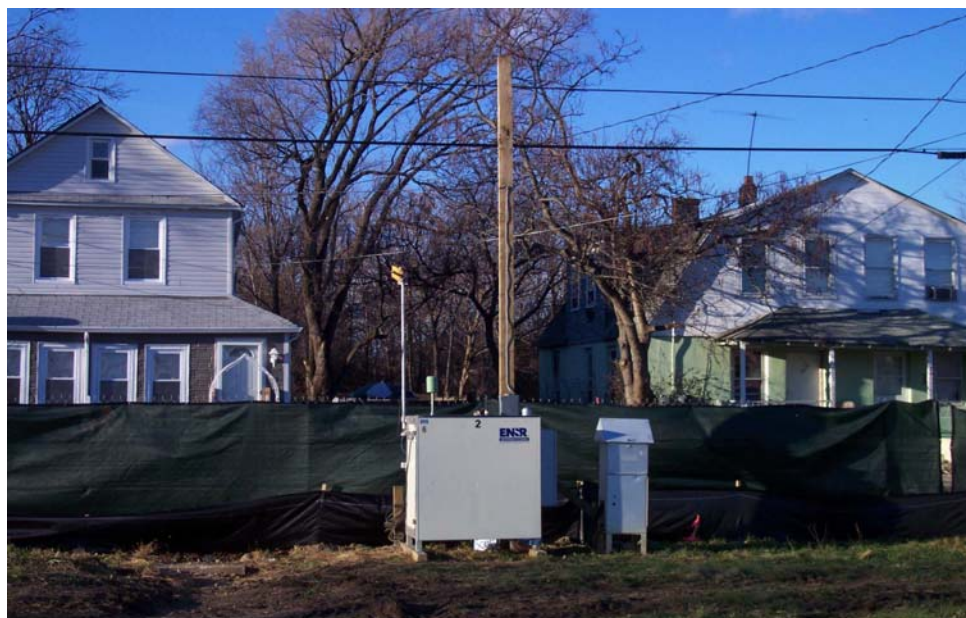
Figure 1. Photograph of typical perimeter air monitoring station used in this case study.
