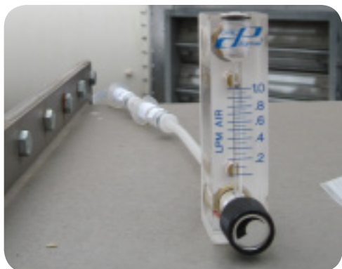
Figure D: Flow is marked by small metal ball. To decrease flow, turn black dial clockwise.
