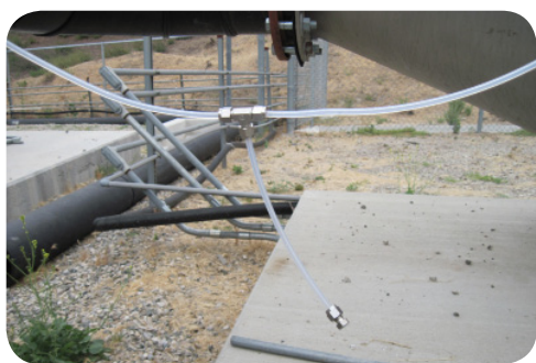
Figure A: One side should attach to gas outlet while the other attaches to calibration tubes.
