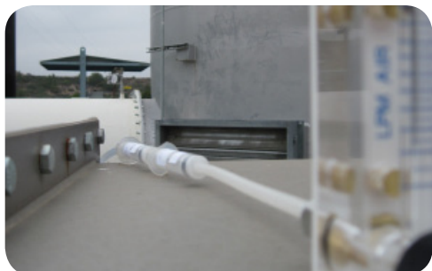
Figure B: Sampling arrows should point toward rotameter. Please note that these figures show two tubes in series. You will only be receiving one tube.
